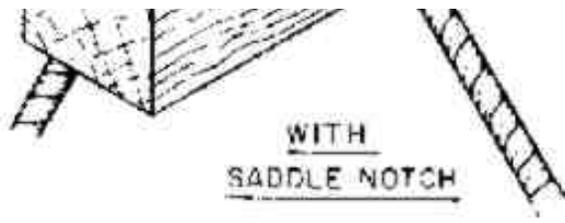
TO PREVENT PULLEY-CORD FROM BEING BURNT BY FRICTION AND BROKEN.
