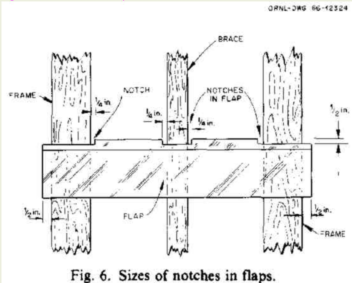
Fig. 6. Sizes of notches in flaps.
