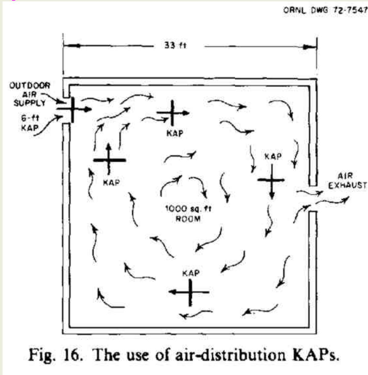
Fig. 16. The use of air-distribution KAPs.
