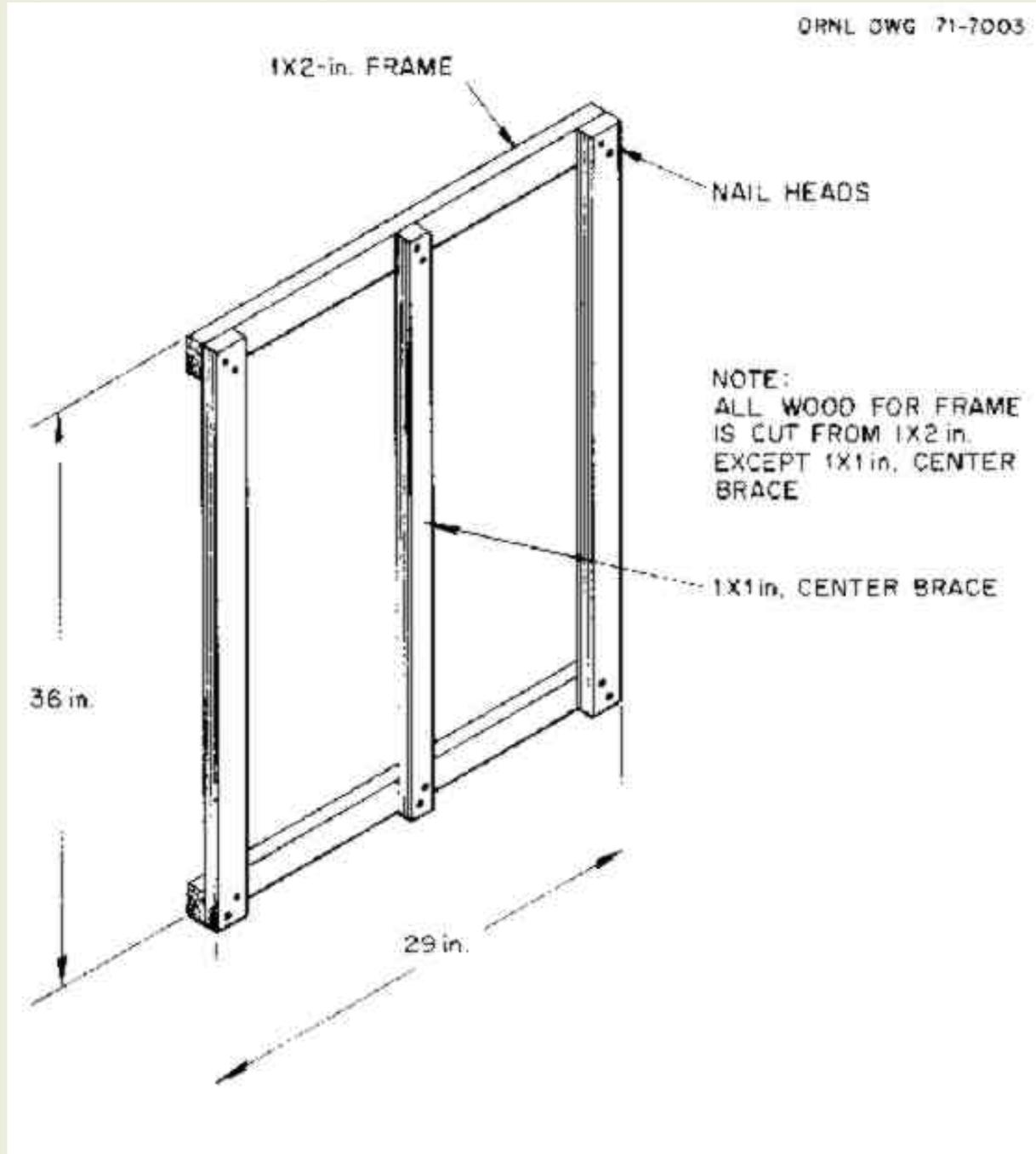
b. To make the front side smooth and flat so that the flaps will close tightly, fill in the spaces as follows: Cut two pieces of 1 X 2-in. boards long enough to fill in the spaces on top of the 36-in. sides of the frame between the top and bottom horizontal boards, and nail these filler boards in place. Do the same thing with a 1 X 1-in. board (or a board the size of that used for the center brace) as a filler board for the center brace (see Fig. 4).
