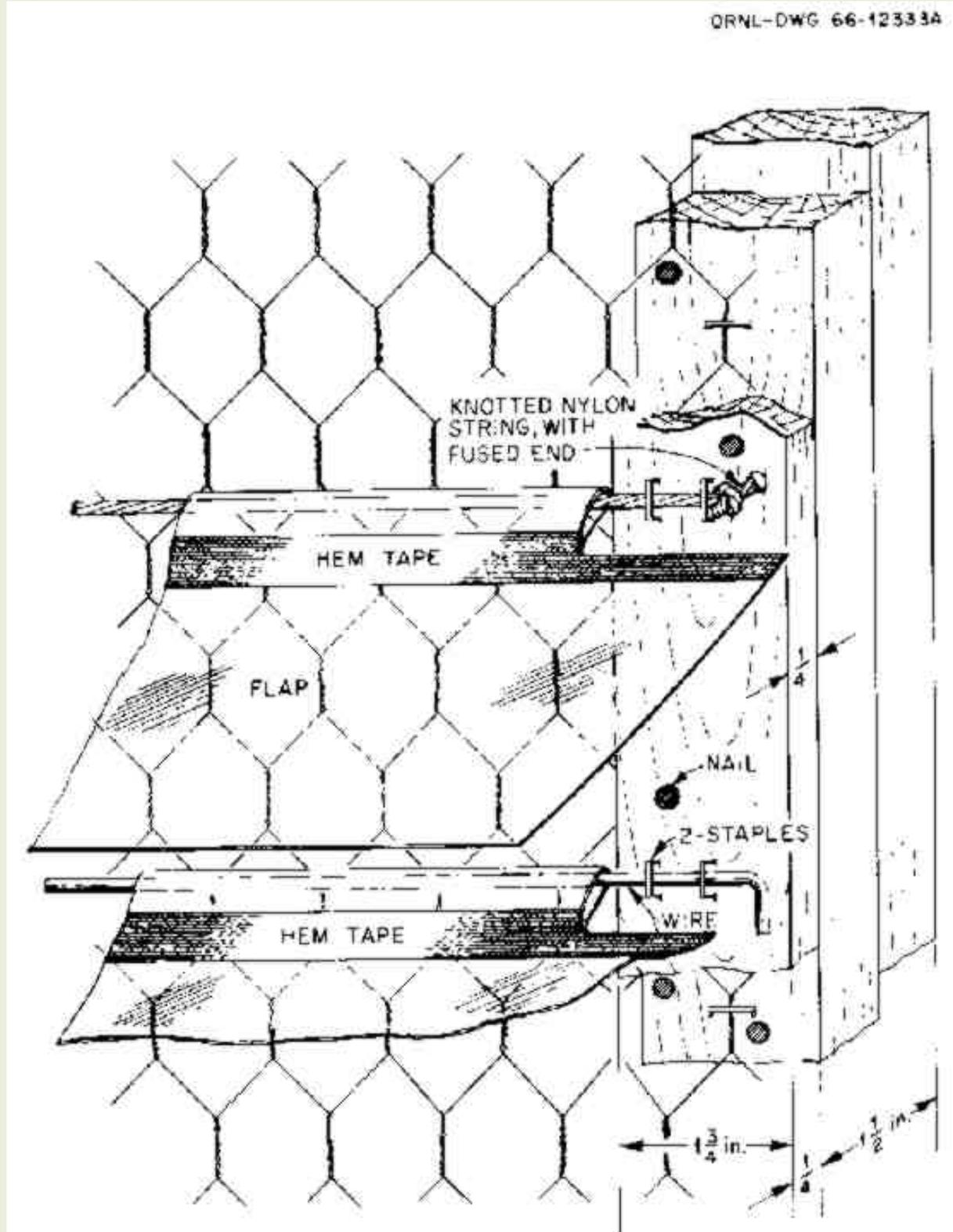
Note in Fig. 13 that each pivot-wire is held firm and straight by 2 staples securing each end. The wire used should be at least as springy as coat hanger wire. If string is used instead of wire, nylon cord about the diameter of coat hanger wire is best for the pivot-strings.
