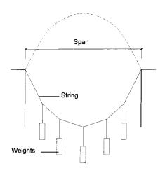
Fig. 1.60 Diagram showing a weighted string describing a catenary curve which, if rotated through 180 degrees, is an appropriate form for a vault of the same span and weight.
