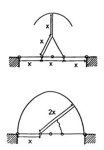
Fig. 1.62 Diagram showing the use of a Y-shaped string to mark out a catenary curve.
