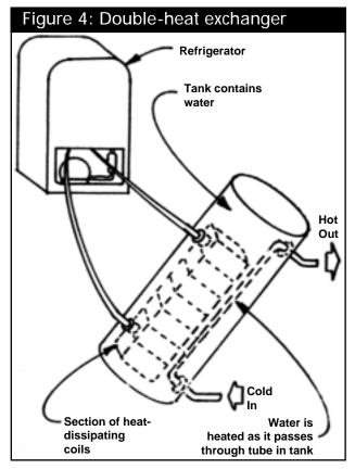
A double-heat exchanger is a safer installation.
