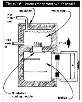
A hybrid refrigerator/water heater built around a solid-state module.
