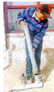
Prototype ram pump in India -- built for one-tenth the commercial price
