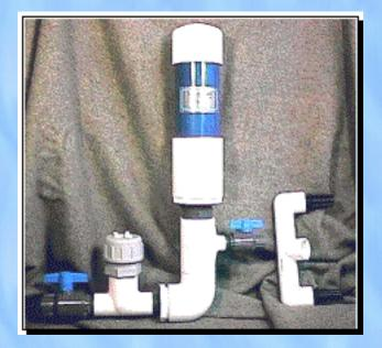
The B & L Ram uses the force of falling water to pump water uphill to where you need it most.... without using any additional source of energy and with only two moving parts. ! As little as a two foot (0.6 meters) fall from the water source to the pump at a flow rate of 3 gallons per minute will drive a small system and provide up to 20 feet of vertical lift to the discharge point.
