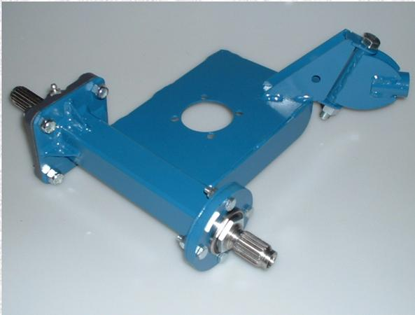
This is a picture of my new pivot weldment. Here you can see the four bolt flange bearing and 6005 bearing for the main shaft support. The flange bearing has setscrews to help locate the shaft. The furling vane pivot has a 1/2" pipe coupling welded on to it to make mounting the vane arm simple. The 6005 bearing sticks out the required .100-.125" to allow the stator to align itself to provide proper clearance to the magnetic hub.
