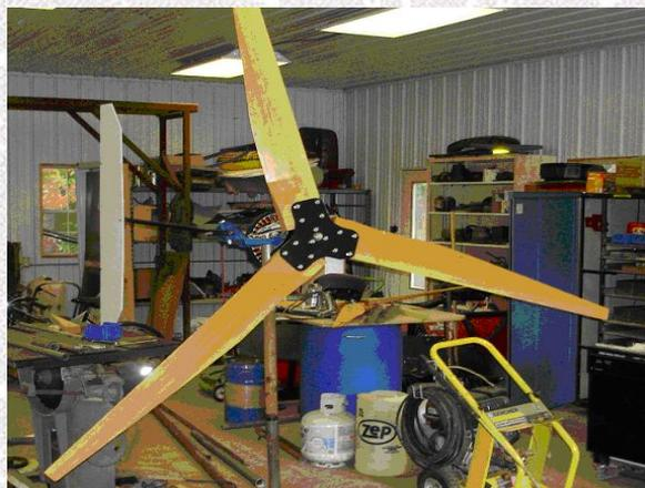
Here is a picture that one of my customers sent to me of his F&P powered windmill. I designed this universal mount to accept one Smart Drive motor. The mount utilizes a Ham Radio antenna rotor bearing. This bearing is heavy duty designed to allow a large Ham radio antenna to rotate. The clamping bolts allow it to be mounted on a mast from 1-1/4" to 2 inch in diameter.
