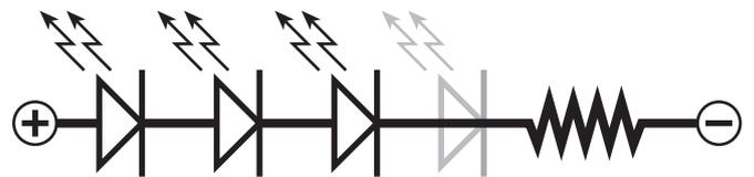
Volts. You can easily construct a series string of many LEDs to run on 12 or 24 VDC. Simply add up the voltage loss of each series junction and subtract this amount from the battery voltage. Divide this figure by junction current and you have the resistance value of
