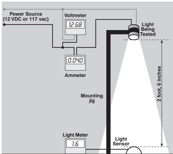
standards have been met. The Greenlee reads out in foot-candles. The distance from the lamp to the light sensor on the Greenlee was 2.5 feet (0.77 meters). I made the electrical measurements (voltage and amperage) using two Fluke 87 digital multimeters.
