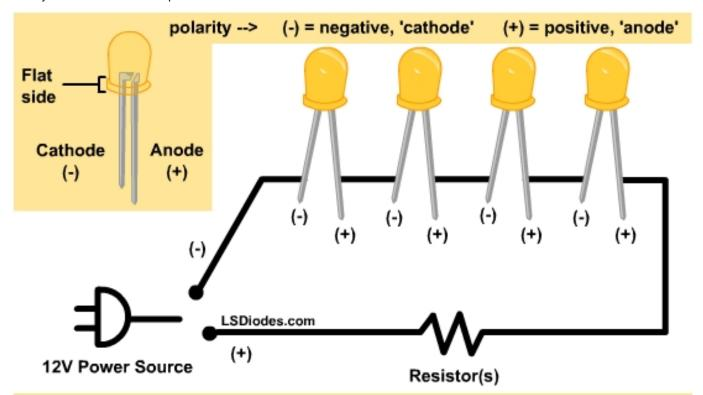
$$\frac{\text{Volts}}{\text{LEDs}} = \frac{12}{4} = 3V$$
