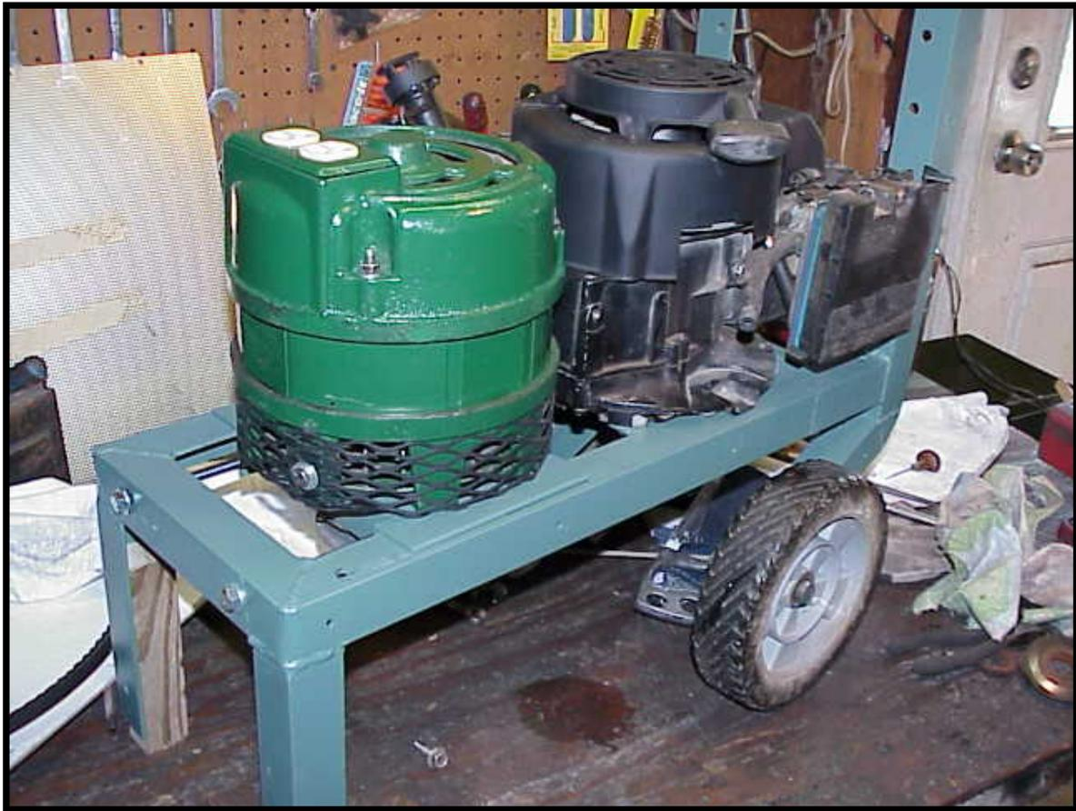
View showing generator slider for belt adjust.
