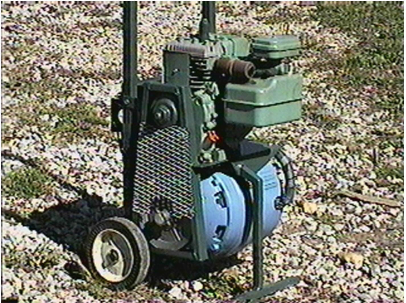
In this view, the belt guard is visible, while the generator is below the engine stand.
