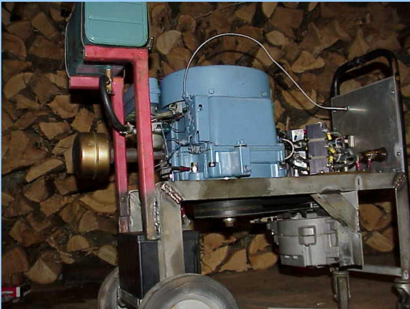
**Another view of the left side. The exhaust pipe is either going to be shielded or moved from under the gas tank for safety reasons.**
