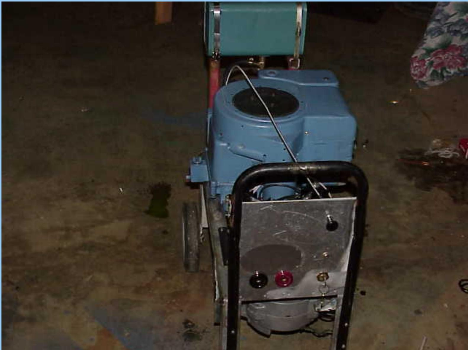
**Here is the front view showing the welding terminals. Black is the negative lead, Red is the positive. The key switch and throttle are also visible.**
