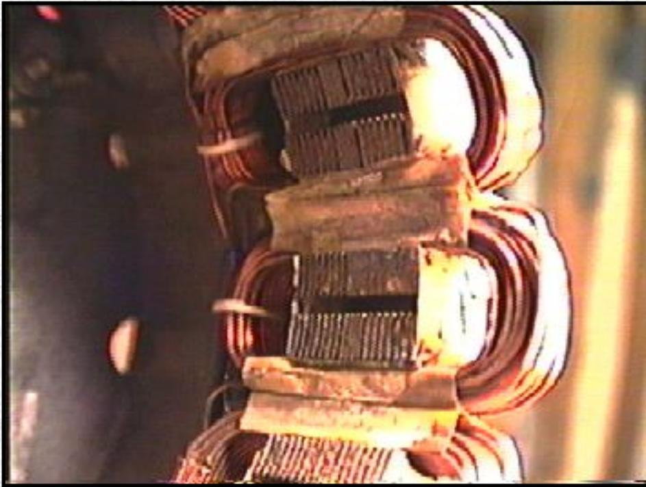
In this close-up shot, notice the two pole faces wound as one and where each third pole has been cut out. A small coil form was made out of plexiglass to wind the coils. I used epoxy glue to hold the coils in place, with fiber tape as an insulator. The coils are about 36 turns of #18 wire, all connected in series.
