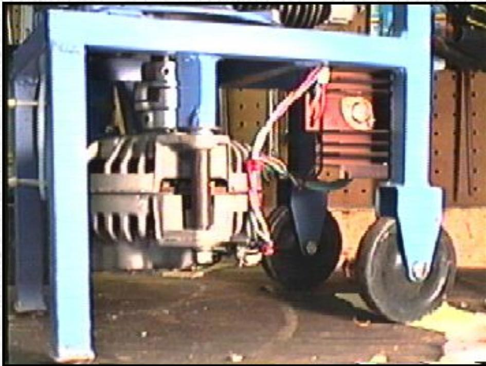
Side view of the alternator, voltage regulator and Lovejoy coupling.
