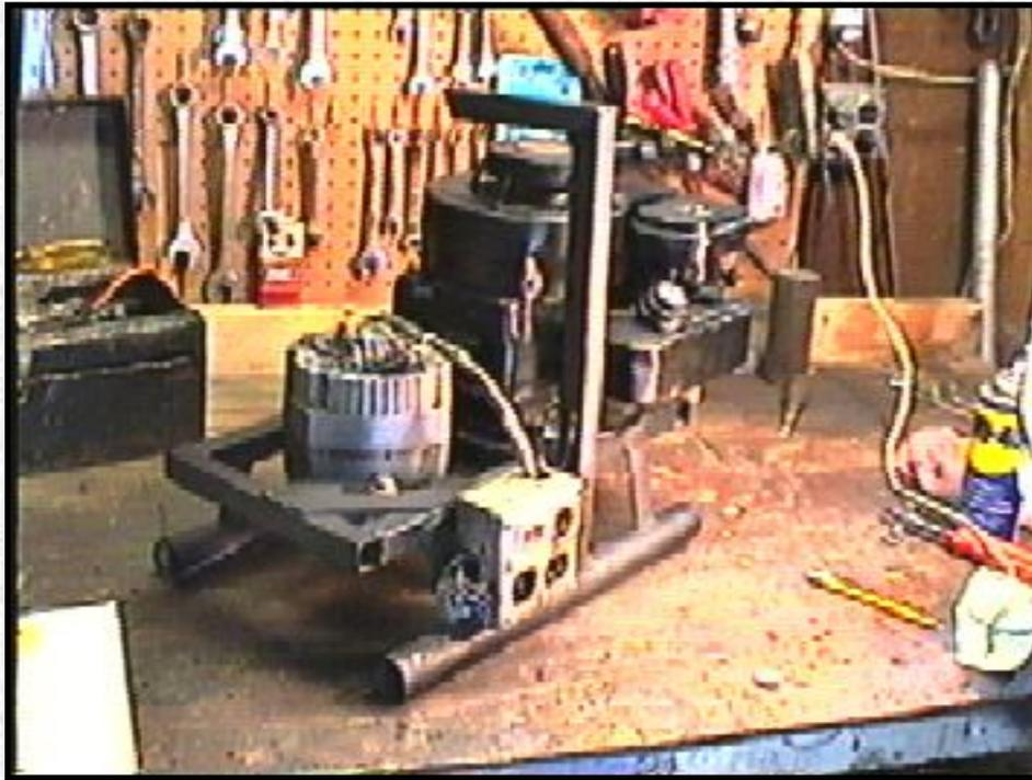
It is capable of 700 watts at 120 Volts AC or DC output. The AC frequency is about 250 to 400 hz, depending of engine speed. You may ask, "What can you power at that frequency?" Plenty! Lightbulbs don't care what frequency they operate at. Devices that are power-transformer operated, such as a radio, TV, VCR, etc. work very well on this frequency.
