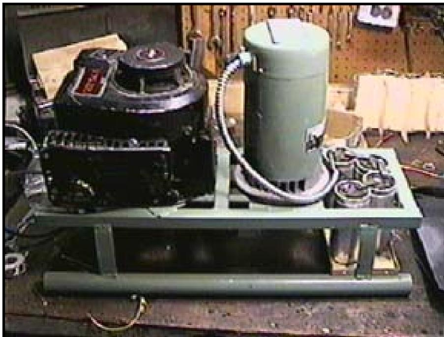
The ex-motor, now an induction generator is driven by a well used 3.75 HP B&S lawnmower engine. A total of 950 watts of lights were ran for about 15 minutes
