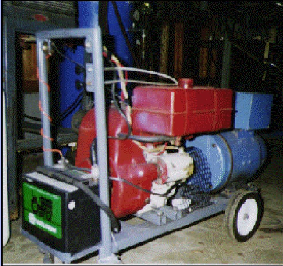
**The** generator that is hooked to this Tecumseh 6 horsepower engine was originally mounted on the faceplate of a Kohler engine. The engine was not hooked to it when I found it at a local junkyard. As a matter of a fact, the rotor and back section were in two different spots in the junkyard! The front plate of the generator, see in the above photo, was supplied and mounted by NJ8V. It was a electric motor faceplate. He manufactured an amazing little alignment ring
