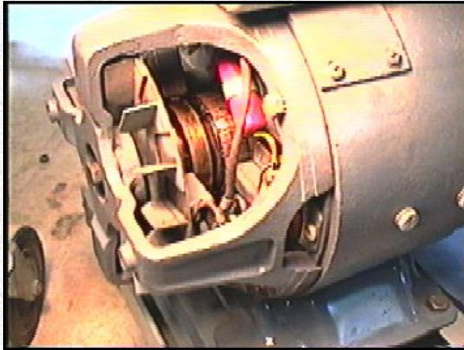
Here are the "innards" of the generator. (Rear shroud removed) Note the AC slip rings (only one is visible), the DC commutator, fan and noise suppressor capacitor.
