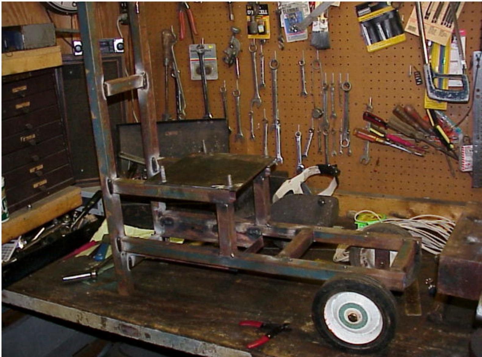
The welded frame before paint...
