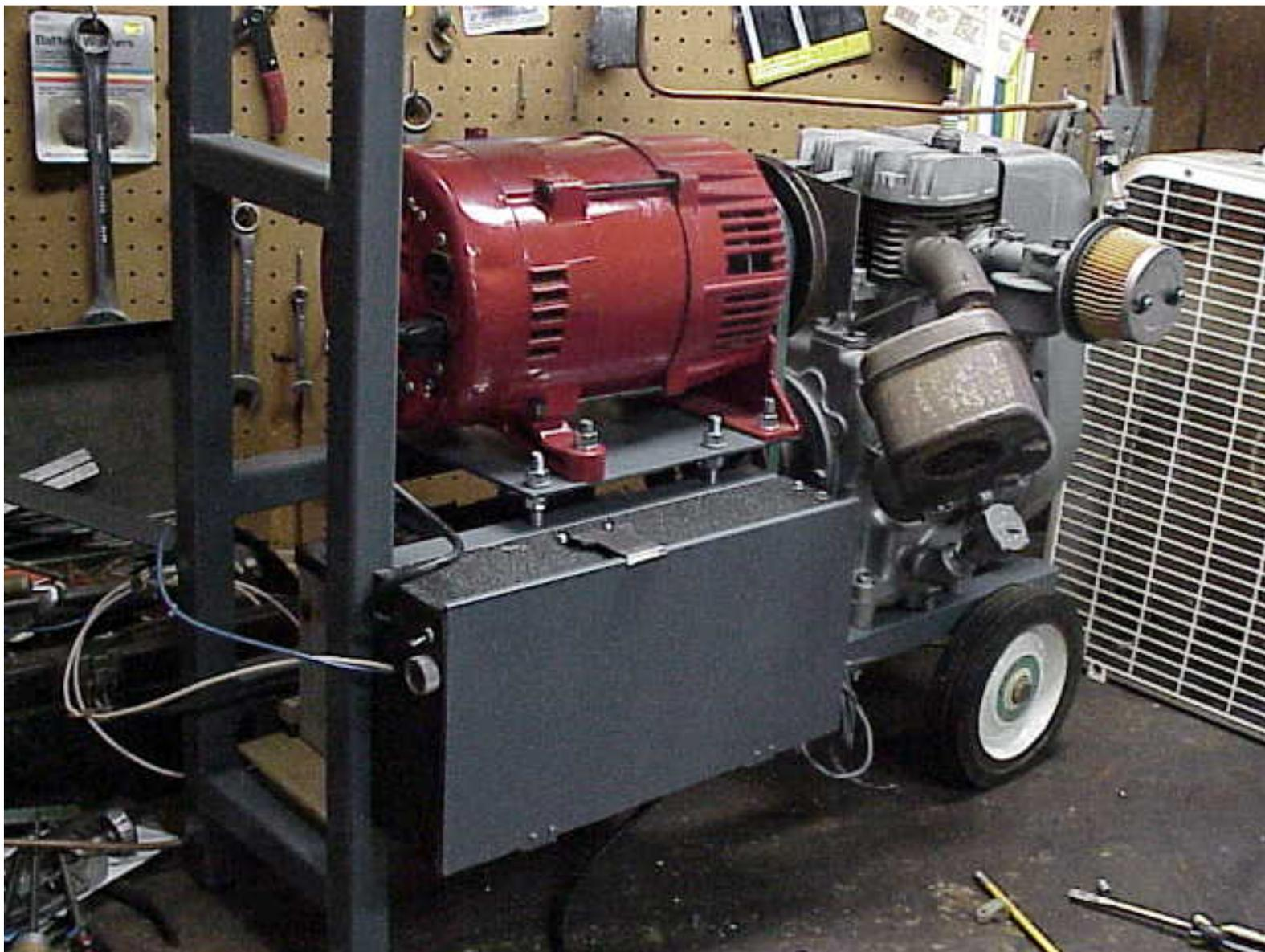
The fun part is attaching the gen and engine to the frame. It's cool when it all comes together! The battery is mounted under the generator and is just visible behind the control box.
