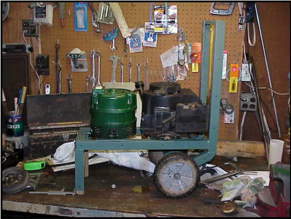
Generator on its new mounting frame with a B&S 5 horsepower
