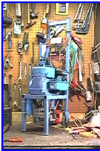
B&S/Chrysler Alternator 12 VDC @ 50 A
