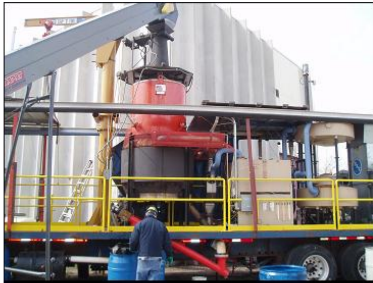
Figure 5: Trailer Mounted 200 kWe Gasifier, FlexEnergy Ltd, 2005
