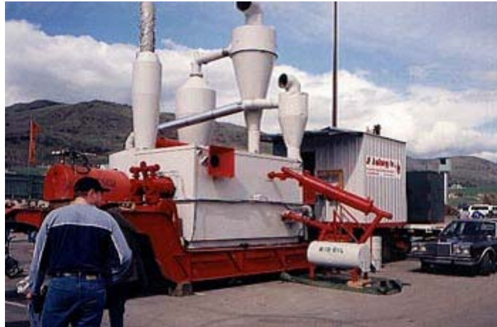
Figure 7: Char and Bio-oil Demonstration Facility 25 tpd (JF Bioenergy Inc.)
