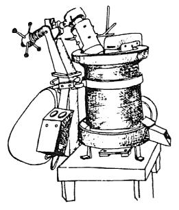
Processes: Oil seeds, nuts Power Source - Capacity: 12-15 kg per charge (several charges per day) Suitable: Large-scale farmer Cost: Rs 7000 India 1985 (US \$ 600) Manufacture Requirements: Castings, machining, fabrication Skill Level: Sophisticated Comments: Also known as rotary oil mills: in power ghanis either pestle or mortar remains stationary while the other rotates (Tools for Agriculture, 1985).
