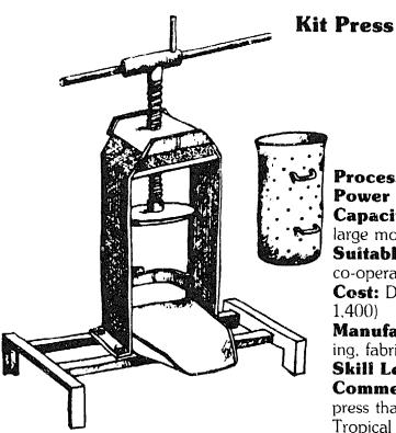
**Processes:** Palm oil mesocarps **Power Source:** Manual **Capacity:** Small model 4.5 kg per press
