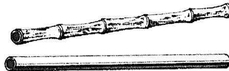
89. The outlet pipe should be long enough to reach through the bottom of the bank from one side to the other. You will need a pipe about 6.5 metres long to reach through the bank at the lower end of your pond.
