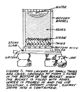
Pile the rocks so that the **flat**, grooved stone rests evenly on top (see Figure 5). Set the wooden bucket on this stone.
