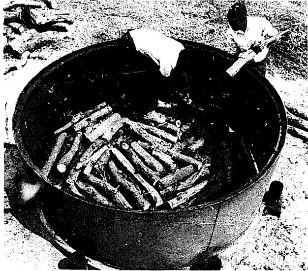
5. Load the bottom section of the kiln with successive layers of wood, filling in as many voids as possible and placing the larger diameter timber towards the centre of the kiln. When the bottom section has been filled roll the top cylindrical section alongside the kiln and push it up on to the supporting rim.
