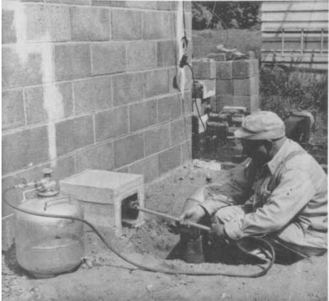
Figure 31. - - Igniting the kiln charge with a torch.
