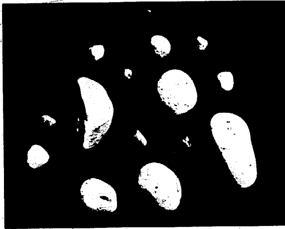
Fig. 4 Very coarse particles of soil.
