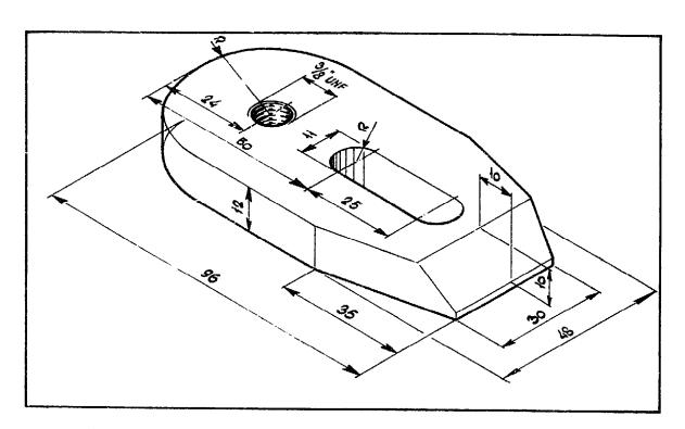
NOTE: tolerance on all dimensions 0,5 mm
