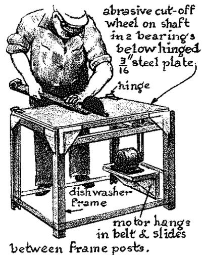
Although high-speed machines may save time, they are also more *dangerous*. After all, we are not in that much of a hurry. Therefore, a one-to-one drive by a secondhand 1750 rpm, 1/4 hp motor will work fine and be *safer*.
