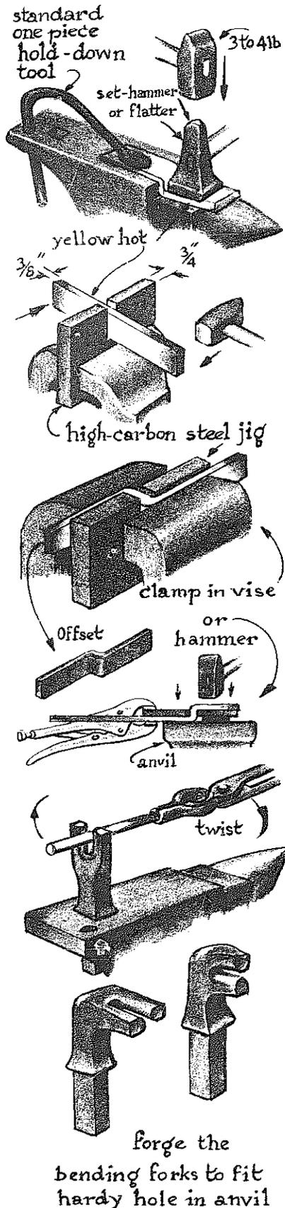
Often offsets must be forged in special hinges, door-bolt receptacles, wall hangers, straps that join boards of different thickness, and so on. To forge an offset bend, proceed as follows. Heat the portion of the bar to be offset to yellow hot and place the bar on the cutoff table so that portion overhangs the table. Fasten the cold part to the anvil with a hold-down tool.
