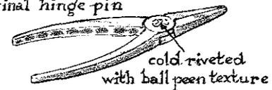
cold riveted with ball-peen texture
