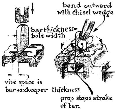
bar folds hot pre-forged keeper-blanks between vise-jaws
