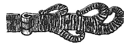
using cross-peen only to shape & texture.
