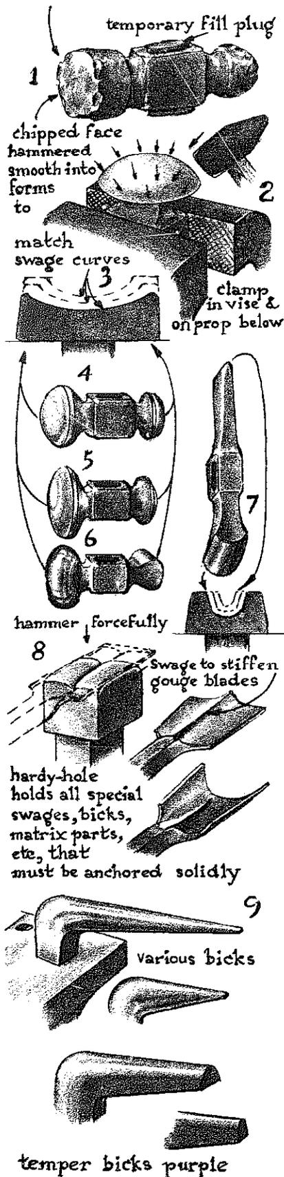
Worn hammers made of good steel may be saved and made usable. Such a hammer, if you find no deep cracks anywhere, can be forged into any specially shaped hammer you may need.
