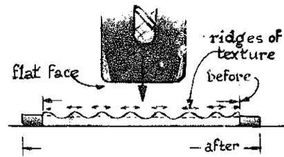
To spread the steel in all directions, first use the ball end of the ball-peen hammer, then the flat end, to spread the steel outward from the center.
