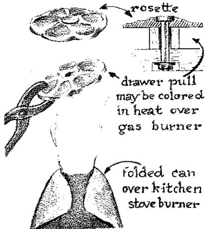
simple decorative forgings from ready scrap-steel items discarded worn automobile engine valves
