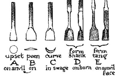
if stock is rectangular bar, its width is to be twice its thickness
