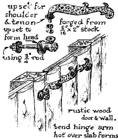
This hinge design can also be used to hang rustic doors and is both strong and practical. The bolt head acts as both bolt part and hinge-bearing socket.
