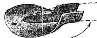
wood handle-end shaped to fit blade-socket
