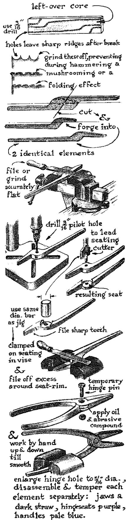
For this pair of  $\frac{1}{2}$ -inch-thick pliers you can use a 4-inch-wide, heavy-caliber leaf of a truck spring.
