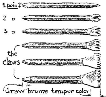
The most commonly used stonecarving tools are simple tools, little changed in design from earliest times. As a rule, stonecarving tools measure about 8 to 10 inches long, and  $\frac{3}{8}$  to  $\frac{3}{4}$  inch thick. All are made from high-carbon steel.
