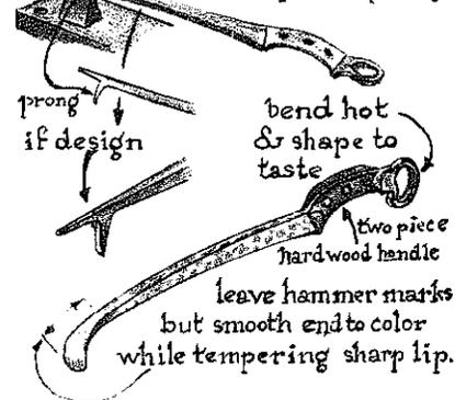
rivet wood sections & rasp, file, sand-down, polish
