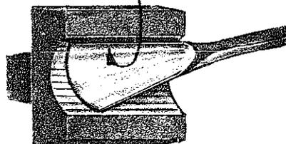
Assume that you have forged the blank with a flat blade. Place this blade in the nearest-size swage groove and gently peen it down without marring its smooth surface. You will notice that during this forming of the blade the thicker part becomes humped up relative to the shank, because it resists the force of the hammer blows. It is this thicker part which now must be hammered down to restore the alignment with the shank.
