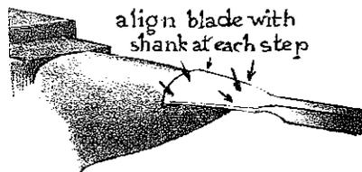
close or open blade curve when needed during refining over horn
