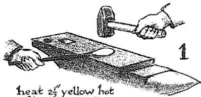
heat 2½" yellow hot & flatten in 1 heat with heavy hammer
