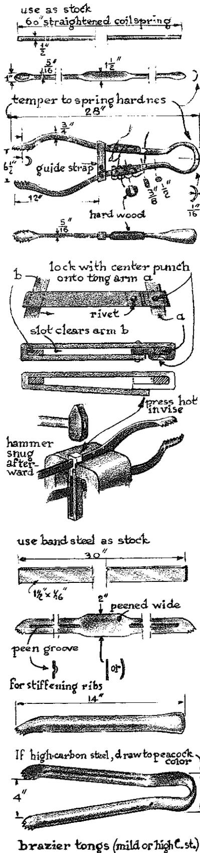
To make a pair of fireplace tongs without hinges, cut a 60-inch length of  $\frac{3}{8}$ - to  $\frac{1}{2}$ -inch-diameter high-carbon steel stock. At yellow heat, forge the middle 8-inch section, peening it out to a width of 1½ inches. This will leave you about  $\frac{1}{16}$ -inch thickness there.
