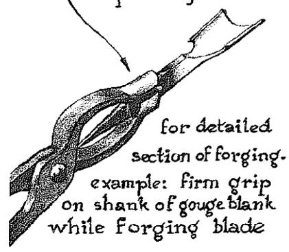
for detailed section of forging.
