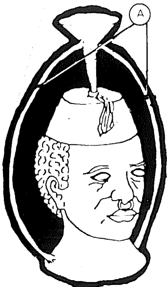
Fig. 38 The addition of runners. A The runners.
