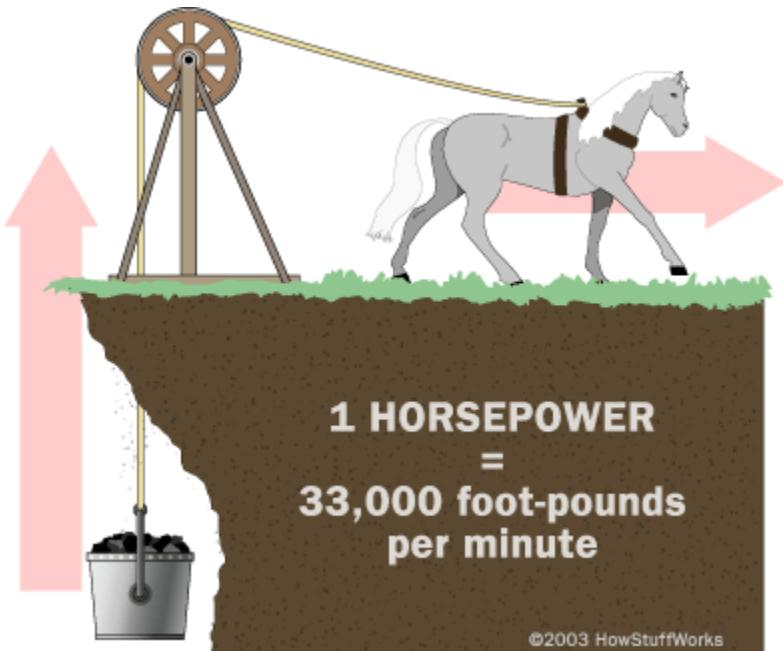
What horsepower means is this: In Watt's judgement, one horse can do 33,000 foot-pounds of work every minute. So, imagine a horse raising coal out of a coal mine as shown above. A horse exerting 1 horsepower can raise 330 pounds of coal 100 feet in a minute, or 33 pounds of coal 1,000 feet in one minute, or 1,000 pounds 33 feet in one minute. You can make up whatever combination of feet and pounds you like. As long as the product is 33,000 foot-pounds in one minute, you have a horsepower.
