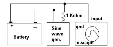
Vary the sine wave source over a range of one to ten megahertz, and look for the peak in the response, showing electrolyte resonance.
