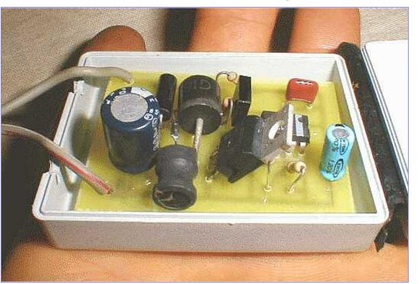
The high power version, for large battery reclaimation, electric vehicle maintenance, high voltage systems, and low level charging. Under development.
