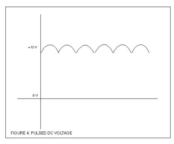
Surprisingly enough, the output of the alternator is not a pure D/C as one might expect, but a pulsating D/C. Because there are three windings, each with a positive and a negative half, by the time the voltage is passed through the diodes, there are six pulsations for each rotation of the rotor. This is close enough to D/C for most automotive components. Critical components, such as radios, have their own internal filtering circuits to further smooth out the waveform to a purer D/C.
