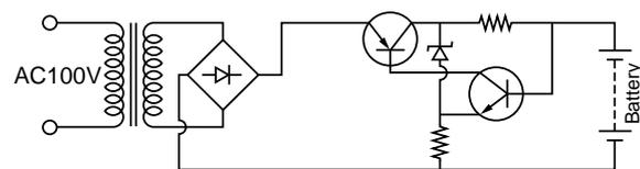
The charging method for the Twicell differs slightly from nickel-cadmium batteries. For this reason, a special charger is necessary. When charging the Twicell, we recommend that you ensure precise charging control, and use constant current charging (quick charging) with a constant current of 0.5 It to 1 It,\*\*\* taking into consideration the various characteristics of the battery. Depending on the model of battery, charging at a constant current equivalent to 0.1 It is also possible.
