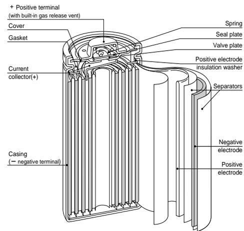
**Fig.5 Internal structure of the Twicell SLIM**
