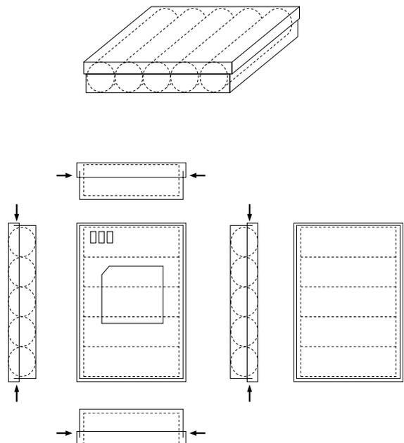
Gas release slits: Where case parts fit together
