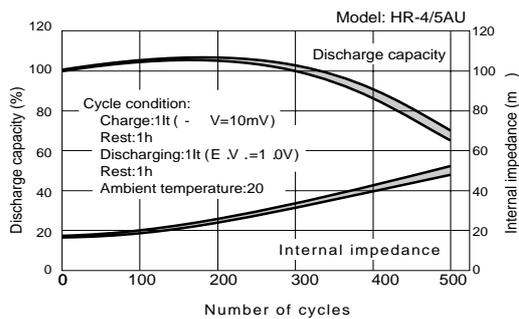
If a battery is charged at a current higher than the prescribed current level, or over-discharged to the point of polarity reversal, or used at low or high temperatures exceeding the recommended range, the charge/discharge cycle life will decrease.
