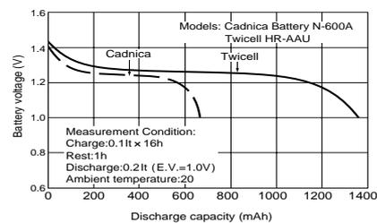
**Fig.2 Charge/discharge cycle characteristics**
