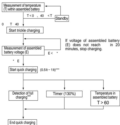
\* .....The value must be determined based on the trickle charging current. As a guideline, use 1.10 V/cell when the trickle current is It/50, and 1.15 V/cell when the current is It/20.
