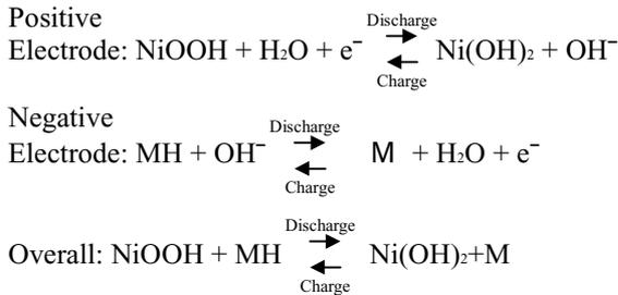
(M: Hydrogen absorbing alloy, MH: Metal Hydride)
