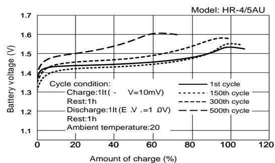
A maximum allowed charging current has been set for the Twicell. If a battery is overcharged and the negative electrode consumes oxygen gas formed at the positive electrode, the hydrogen absorbing alloy will become partially oxidized and will deteriorate the performance of the negative electrode. Therefore, when charging the Twicell it is necessary to avoid over-charging as repeated overcharging shortens battery service life.
