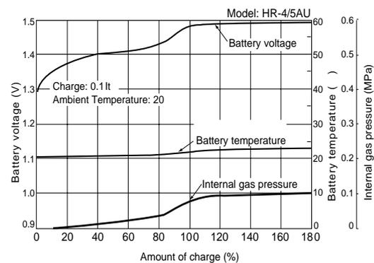
Also, as there is a limit to the negative electrode's ability to consume oxygen gas formed at the positive electrode due to over-charging, a maximum allowed charging current has been set to assure a balance between the amount of oxygen gas formed and the negative electrode's ability to consume it.
