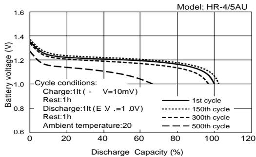
If the Twicell is repeatedly subjected to deep discharge accompanied by polarity reversal, as described previously, battery service life will decrease. For this reason, it is necessary to avoid over-discharging.
